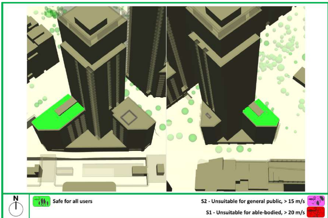
Safety Ratings – LVL 11 Roof Terrace
