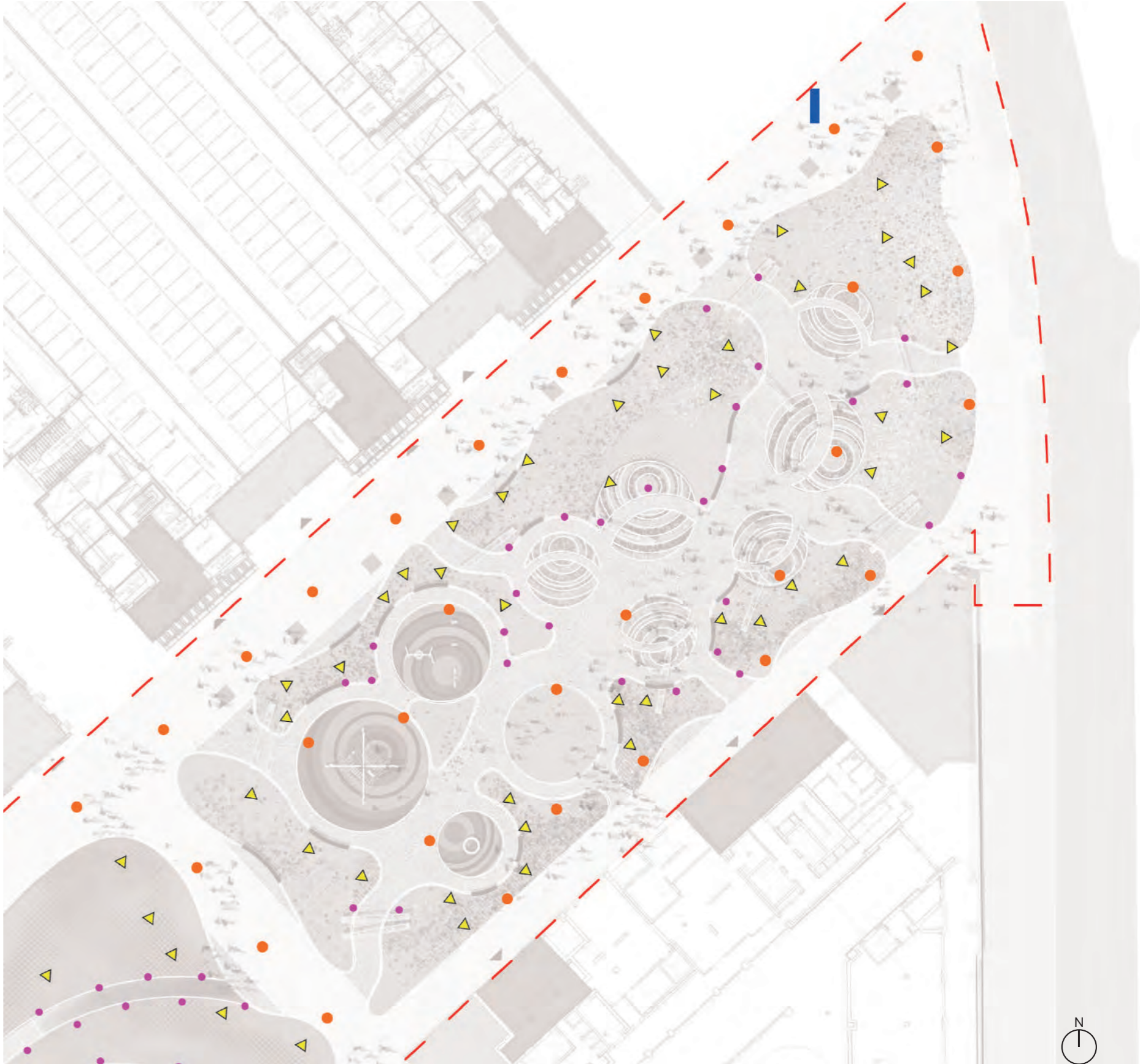
Figure 146. Diagram showing lighting location in Belvedere
