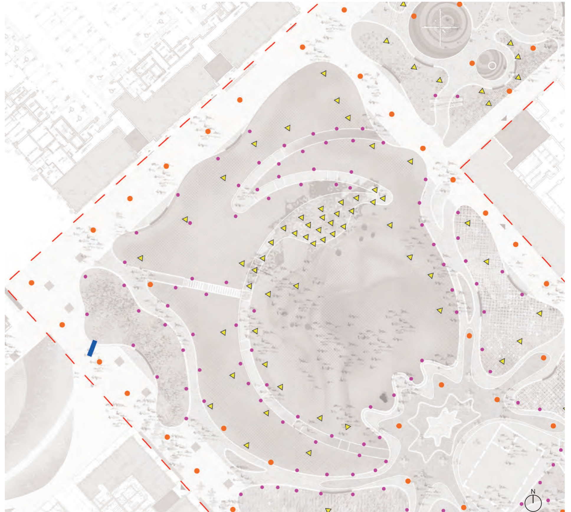
Figure 142. Diagram showing lighting location in Victory Park
