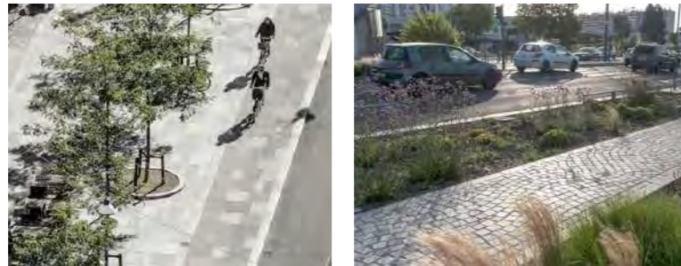
Rather than a traditional treatment, subtle paving changes demarcate the cycling route.
