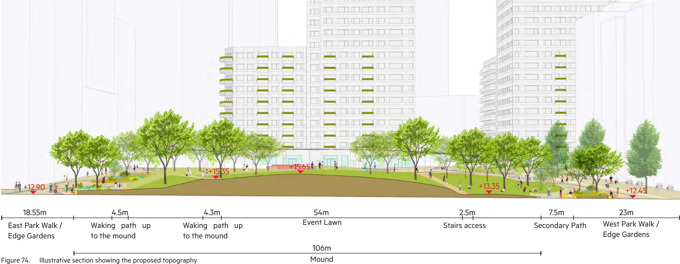
Figure 74. Illustrative section showing the proposed topography
