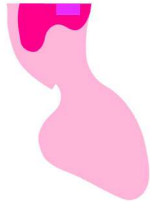
Figure 170. Total Area: 250 sqm. Pink indicates the total area covered by a canopy, with purple indicating the 11% dedicated to the counter, back counter, storage, and servicing. The magenta (15%) indicates the enclosed seating area.
